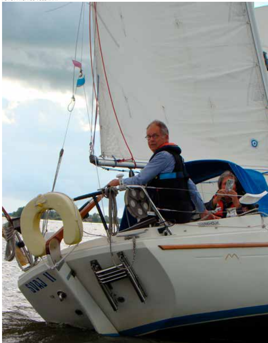
The swimming ladder is tightly attached to the stern.
